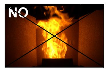
**NON OPTIMAL** combustion, the flame is high and weak and is of an intense orange colour also a large amount of unburned pellets are left over inside the burner.
