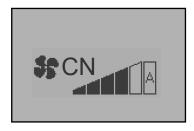
When the room temperature reaches the set value (SET ROOM TEMP), the stove goes into Normal Modulation, the front F fan runs at minimum speed and the CN fan continues to run independently depending on the set power level (CN).
