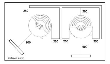
Caution: For some models the minimum safety distance from flammable materials may be different than those shown in the figure below. Therefore, always refer to the product identification plate generally located on the back of the stove to ensure minimum safety distances for the specific model.
