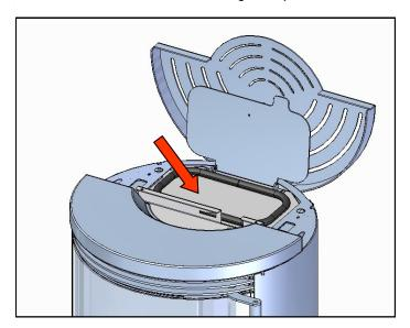
Use only wooden pellets with a 6 mm diameter and 30mm maximum length, EN PLUS certified class A1.
