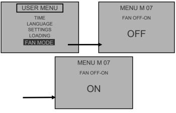
Allows to use the relax mode with installed ducting for HYBRID stoves: <u>Compact, Aladino, Clessidra, Dream, Elegance, Ergonomic</u>. Fan deactivation works for the power P1, P2,P3, while the power P4 and P5 the fan works automatically.
