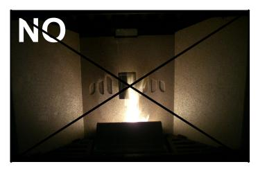
**NON OPTIMAL** combustion, the flame is too stretched and a large amount of burning pellets are blown out of the burner.
