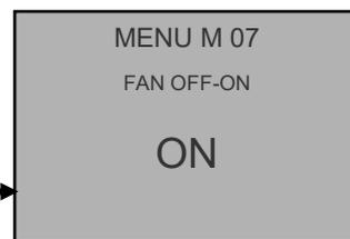
Allows to use the relax mode with installed ducting for **HYBRID** stoves: Compact, Aladino, Clessidra, Dream, Elegance, Ergonomic. Fan deactivation works for the power P1, P2,P3, while the power P4 and P5 the fan works automatically.
