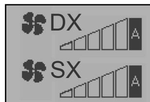
When the room temperature reaches the set value on the stove (SET ROOM TEMP), the stove goes into Modulation and the fans (F, DX, SX) run at minimum speed.
