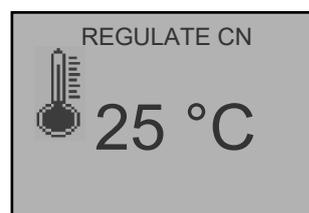
When the room temperature reaches the set value on the stove (SET ROOM TEMP), but not the SET temperature for the CN fan (REGULATE CN), the stove continues to operate at its set power (POWER SET), the F fan runs at minimum speed and the CN fan continues to run at the set power level on the stove.
