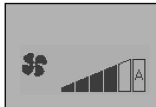
If **A** (Automatic) is set, the heating fans will work at a set speed depending on the selected combustion power level.
