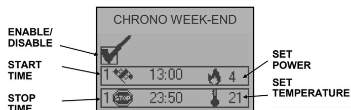
It is possible to set the time frames defined by the set times where the **OFF** setting means the clock will ignore the signal.
