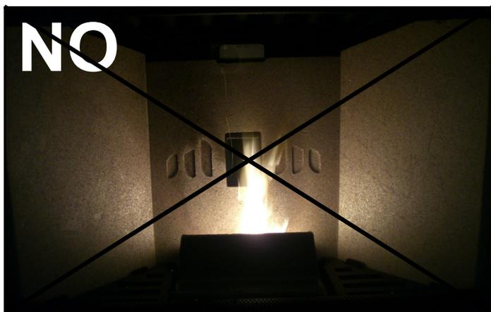
**NON OPTIMAL** combustion, the flame is too stretched and a large amount of burning pellets are blown out of the burner.
