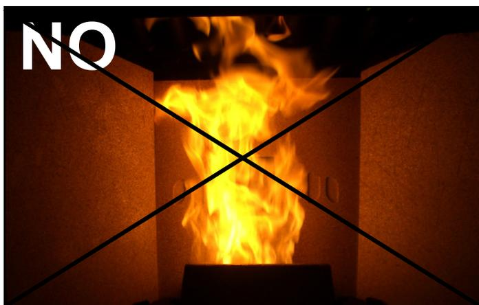
**NON OPTIMAL** combustion, the flame is high and weak and is of an intense orange colour also a large amount of unburned pellets are left over inside the burner.
