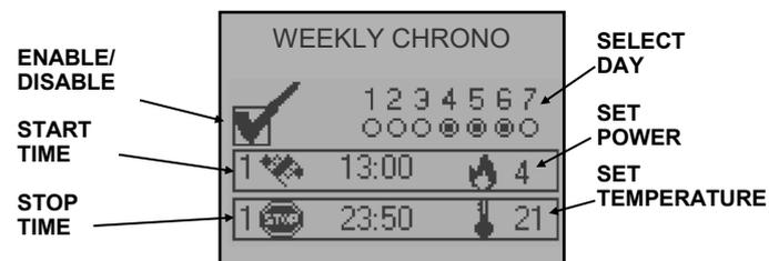
It is possible to set the time frames defined by the set times where the **OFF** setting means the clock will ignore the signal.
