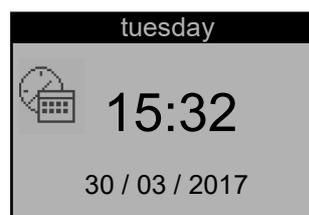
The control unit is equipped with a lithium battery which allows the internal clock to have an autonomy for more than 4/5 years.
