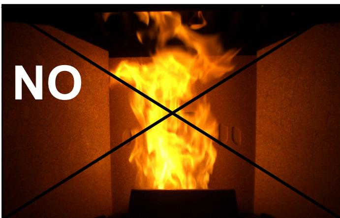
NON-OPTIMAL combustion, the flame is high and weak and of an orange color with a high quantity of unburnt pellets in the brazier.
