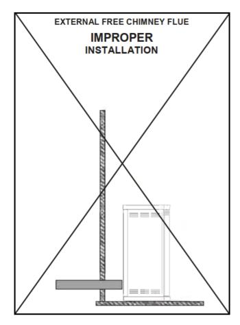
For the connection to the chimney, we recommend the use of stainless steel pipes in compliance with current regulations, without reductions, and with a maximum inclination of 45 °. It is recommended not to use flexible metallic and / or fiber cement materials.
